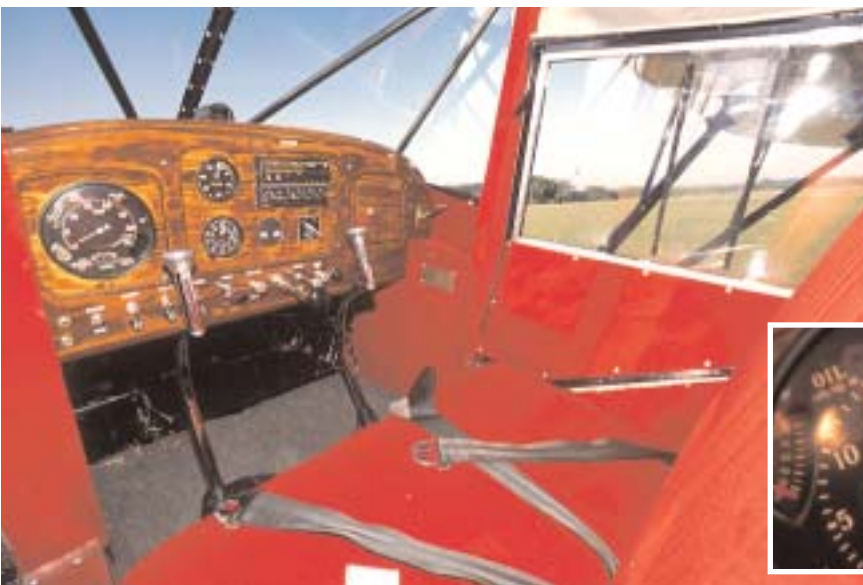
The multifunction tachometer dominates the left side of the instrument panel in the Rearwin. All engine conditions are indicated within the dial of the tachometer. Oil temperature and pressure, fuel quantity and pressure, and an ammeter to monitor the electrical system.
