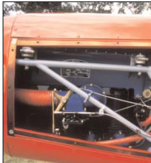
The Fairchild 22 originally had, among a couple of choices, the Menasco C-4 engine; but the engine that came with the project was the later model D-4, complete with enclosed rocker boxes. Al Ball overhauled the relatively rare engine.
