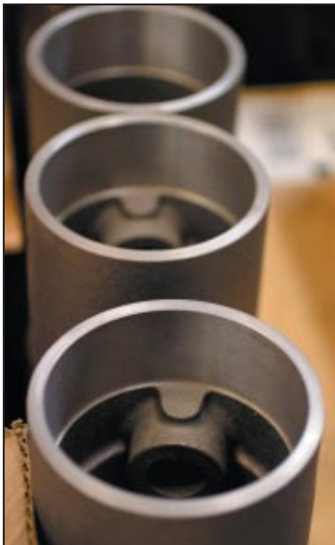
The cast iron pistons slip into cast iron cylinders, which are screwed into the cast aluminum crankcase.
