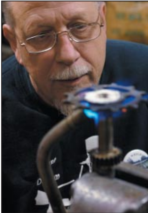
Using a rosebud tip on his torch, Steve Hay heats up the sprocket for the valve camshaft in preparation for silver soldering.
