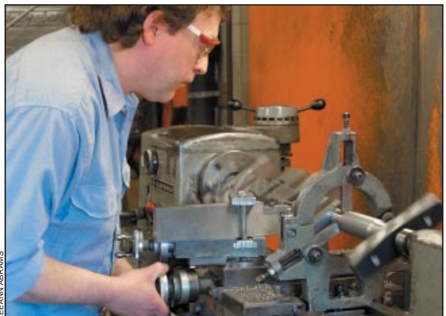
Using a lathe, Mike Newberg turns the raw crankshaft, which was drilled out from a steel blank.
