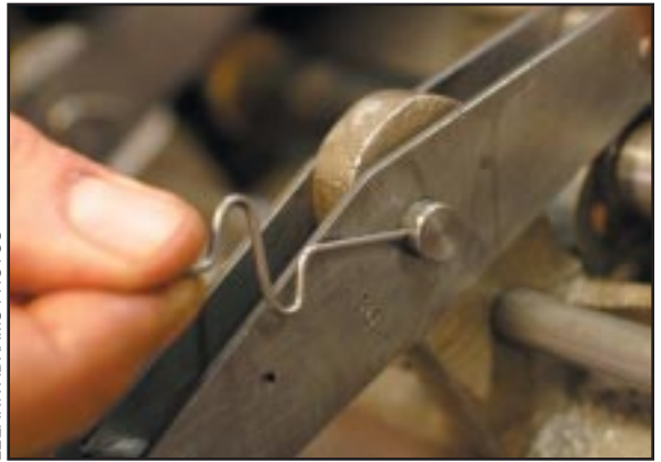
Every aspect of the first Wright brothers' engine built by Charlie Taylor is exactly duplicated, including the open rocker arms, which are built up using sheet steel. The spring steel keeper is positive acting, yet it allows quick disassembly when needed.
