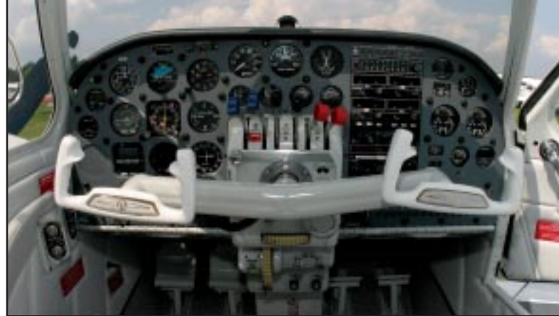
Since the original panel had patches screwed to patches, the entire panel was redesigned and a new one fabricated. Behind the panel and throughout the airframe, the wiring harness was replaced, removing pounds of unused wiring left from previously installed instruments.
