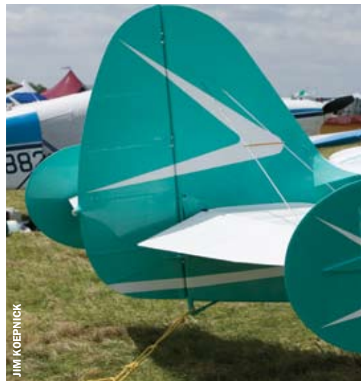
The distinctive triple tail of the Bellanca 260.
