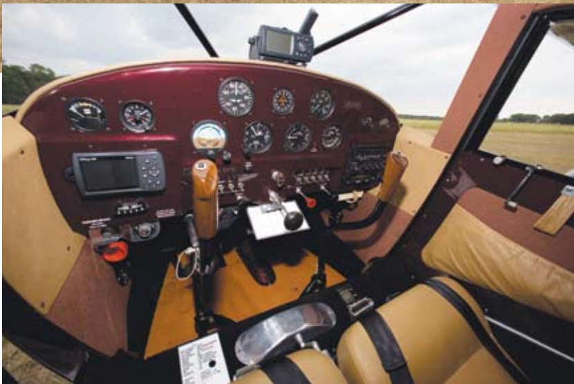
These two views of the cockpit show the care that went into the fit and finish of the entire project. The seats are Tempefoam covered in Connelly leather. Duane says he started with the instrument panel's layout and rebuild, and then restored the Luscombe around it.
