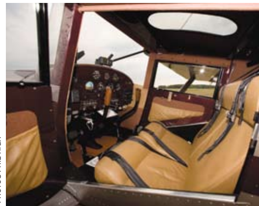
These two views of the cockpit show the care that went into the fit and finish of the entire project. The seats are Tempefoam covered in Connelly leather. Duane says he started with the instrument panel's layout and rebuild, and then restored the Luscombe around it.
